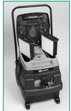
Filters mounted parallel to motor to maximize tank space. Located above dust and water levels to maintain maximum air flow and suction.
