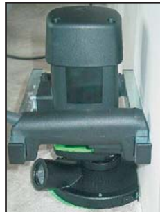
Removable front dust guard for grinding up to walls and edges.
