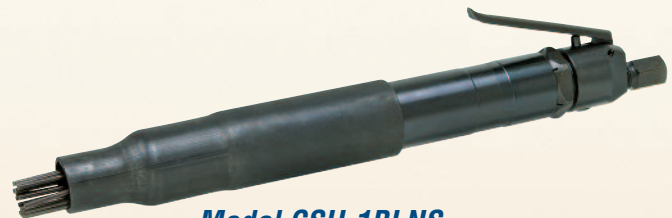
Model CSU-1BLNS Needle Scaler with Lever Throttle Non-sparking CuBe needles (Ex308-319B) available.
