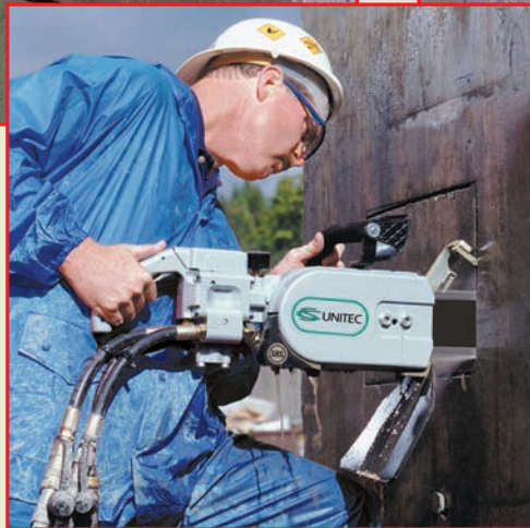
Above: Optional SpeedHook® guides saw for straight cutting (see page 30).
