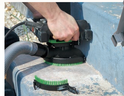
EBS 125 Concrete Grinder (10,000 RPM) Perfect for concrete surface preparation and smoothing.
