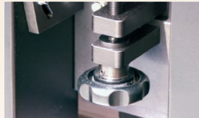
The disc wear is adjusted using a hand wheel with a threaded spindle. The face angle can be adjusted using a motorized system.
