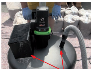
Pouring inlet tube and integrated dust extraction port reduce airborne dust while adding and mixing materials
