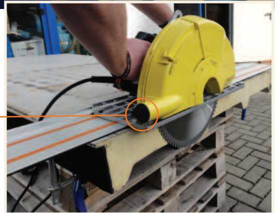
Integrated dust collection port
