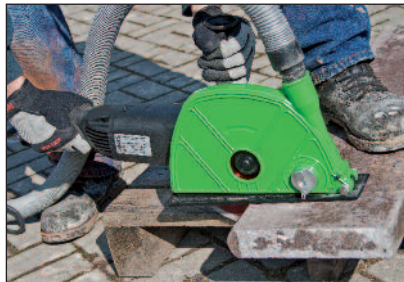
Vibration-dampened, repositionable handle for left- or right-handed use
