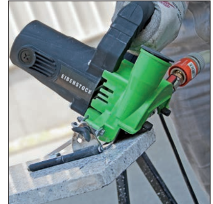
Stepless mitre adjustments up to 45° – without tools
