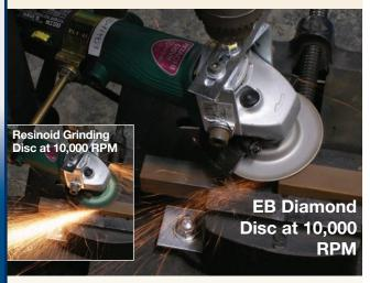
EB diamond grinding discs reduce sparking up to 1/100 of that produced by resinoid grinding wheels (inset left).
