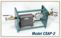
Removes moisture and dirt from air lines; a float valve automatically ejects water and dirt
