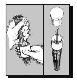
Hold the needles loosely and shake the holder, needles will fall into location holes The correct position of parts when changing needles
