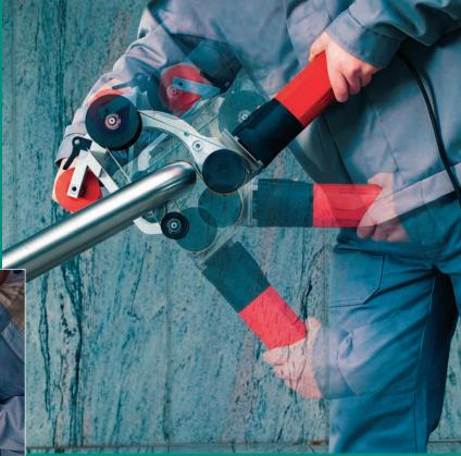
The LRP 1503 BOA Pipe Sander is the perfect solution for sanding and polishing pipe constructions. The sanding arm snakes up to 270° around the radius of the pipe. The operator simply rotates the BOA slightly to achieve a full 360° finish. Spring resistance between the deflection rollers ensures that the sanding arm and belt are always uniformly tensioned. The BOA saves time finishing stainless steel and other ferrous and nonferrous pipe.
