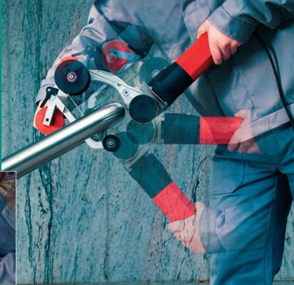
The LRP 1503 BOA Pipe Sander is the perfect solution for sanding and polishing pipe constructions. The sanding arm snakes up to 270° around the radius of the pipe. The operator simply rotates the BOA slightly to achieve a full 360° finish. Spring resistance between the deflection rollers ensures that the sanding arm and belt are always uniformly tensioned. The BOA saves time finishing stainless steel and
