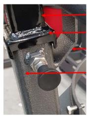
Larger square profile motor mount (p/n PH606) with splash protection shroud
