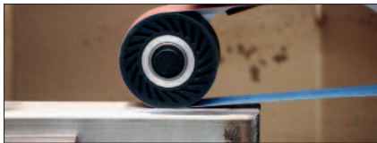
1 Gas pressure cylinder allows belt to conform to contour of pipe with proper pressure.
