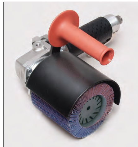
1 HP air motor at 90 PSI
