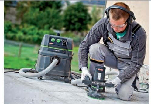
**Activate vacuum on/off from power tool controls**
