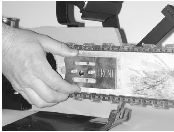
STEP 6 Install bar clamp plate over the bar studs.
