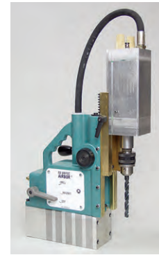
With a geared chuck adapter (Part No. IBC 18) and extra rack (Model No. AB-4300-2R), AIRBOR™ easily converts to a standard drill press with a 7 1/2" stroke.
