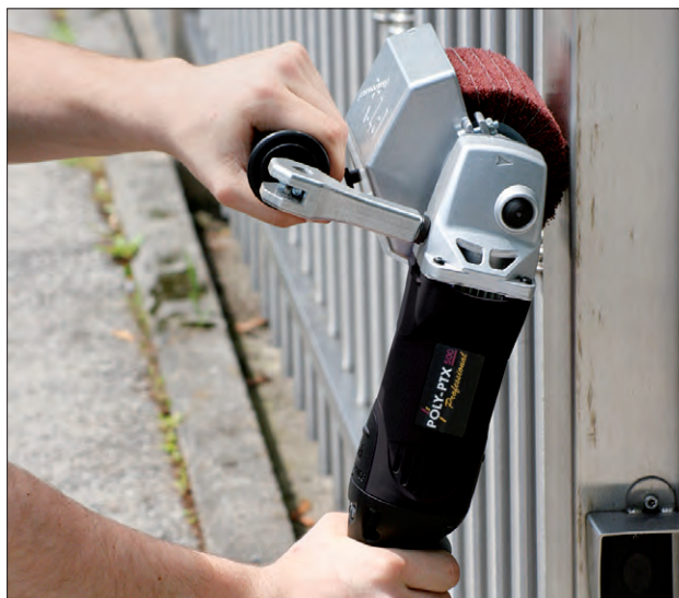
Satin finishing using interleaf fleece wheel.
