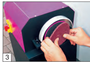
3 Uses the FIX HOOK AND LOOP SYSTEM (See pages 105-107). For replacement flap discs, see page 93.
