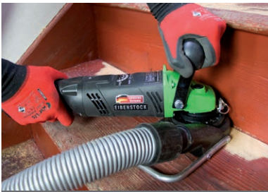
Carbide milling disc for wood surfaces (P/N 37124)
