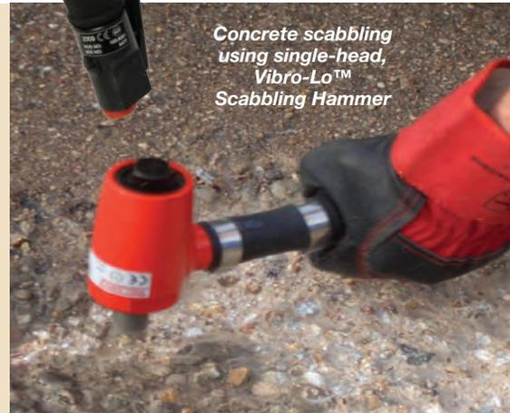
Concrete scabbling using single-head, Vibro-Lo™ Scabbling Hammer
