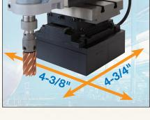
Model MAB 825 KTS features multiaxis positioning, allowing the drill to be adjusted up to 4-3/4" forward/ backward and up to 4-3/8" left/right after magnet is adhered to surface. Ideal for job site drilling, boring and slotting applications where dismantling is not feasible.
