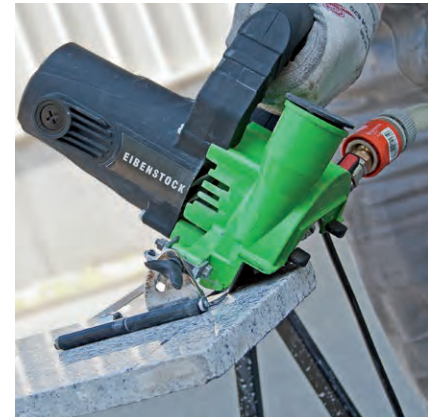
Stepless miter adjustments up to 45° – without tools
