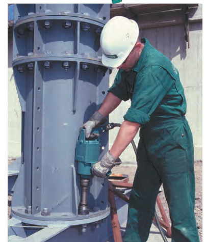
6 1515 0010 3/4" Hydraulic Impact Wrench 1220 ft.-lbs. torque
