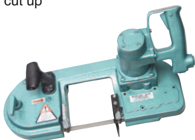
Deep Throat™ AirBand Model 5 6031 0010 – 7" OD cutting capacity ATEX Classified for Ex Zone 2
