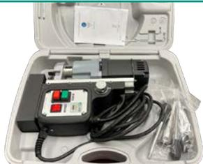
**Standard Equipment** includes manual chuck with set screws, safety chain, carabin hook, allen keys, and carrying case. (CSU 50S shown)
