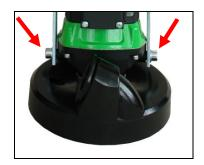
Screw on the switch-box with the 4 cap nuts (M 5).
