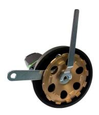
Push the protection hood as far as upwards that you can put the jaw wrench, size 32 (1) between gearbox and grinding wheel on the keyholes of the driving disc.
