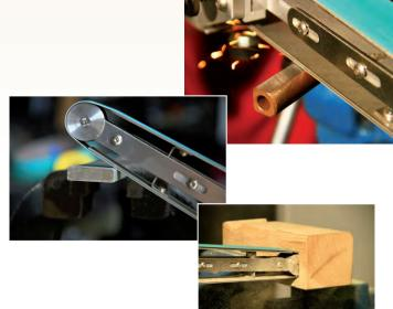
Convert the Gladius® 1800 to a benchmounted grinder with optional machine stand for precision grinding and polishing. Optional machine stand: Part No. 38660
