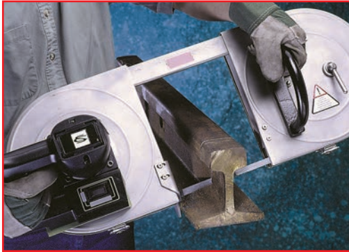
Electric Deep Throat™ Model 5 6040 0010 cuts a section of rail
