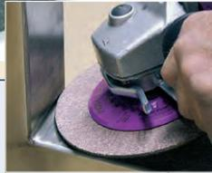
Obtaining good polish quality when finishing corner welds is difficult, especially for the fabrication of railings. The POLY-MAGIC-WHEEL was designed to help you more easily produce a truly perfect finish in these applications. This highly compacted fleece disc was designed specifically for grinding and polishing bead and corner welds. The POLY-MAGIC-WHEEL disc can reduce the time required for this work to a minimum, and the result can only be described as a minor miracle.
