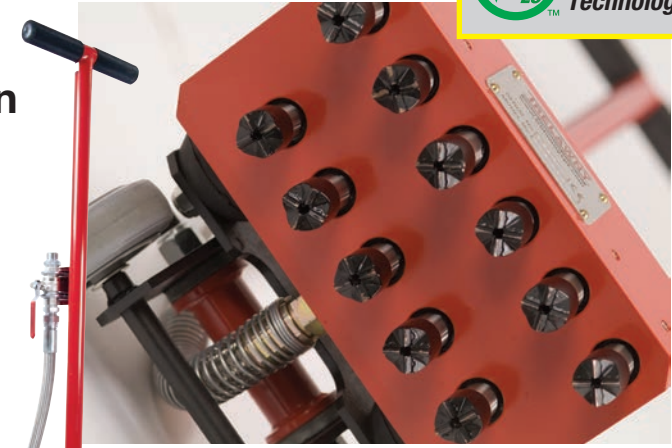
11 heads provide 33,000 BPM (11 x 3000 BPM)
