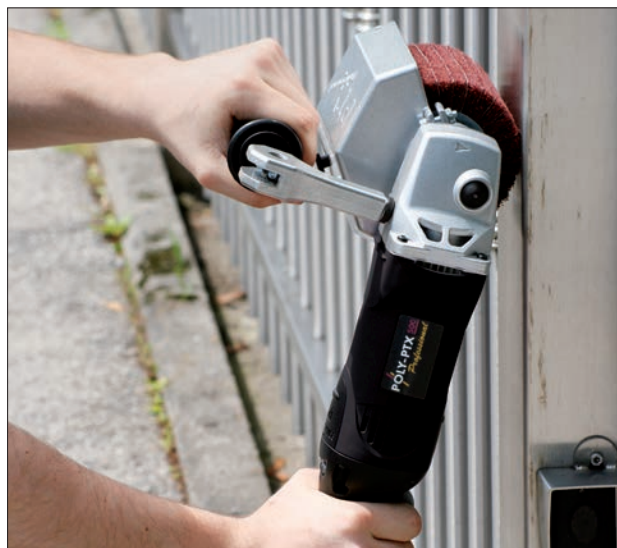
Satin finishing using interleaf fleece wheel.
