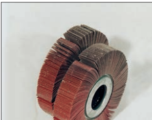
Spare flap wheels for sheet metal deburring machine BE 5 Grit 40, 60, 80, 120
