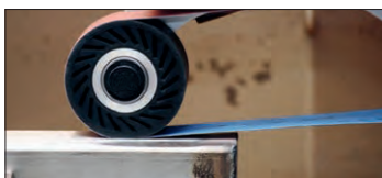
1 Gas pressure cylinder allows belt to conform to contour of pipe with proper pressure.
