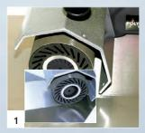
Step 1 - Pre-grinding Prepare with TZ Pyramid sleeve grit A45 (possibly A65) to remove mill skin, scratches and minor unevenness.
