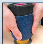
To remove the grinding sleeve, place the expansion roller on a round object that is slightly smaller than the roller. Then push the sleeve down slightly using both hands.
