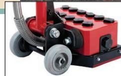
Optional dust shroud, P/N 437.0100, to collect dust and debris when connected to a dust collection vacuum.
