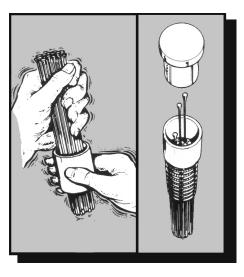
Hold the needles loosely and shake the holder, needles will fall into location holes
